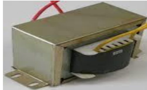
Fig 5: Step down Transformer
