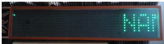
Fig 9: LED Dot Matrix Display
